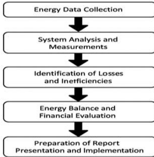
Figure 5.5 Detailed Energy Audit Process Flow
