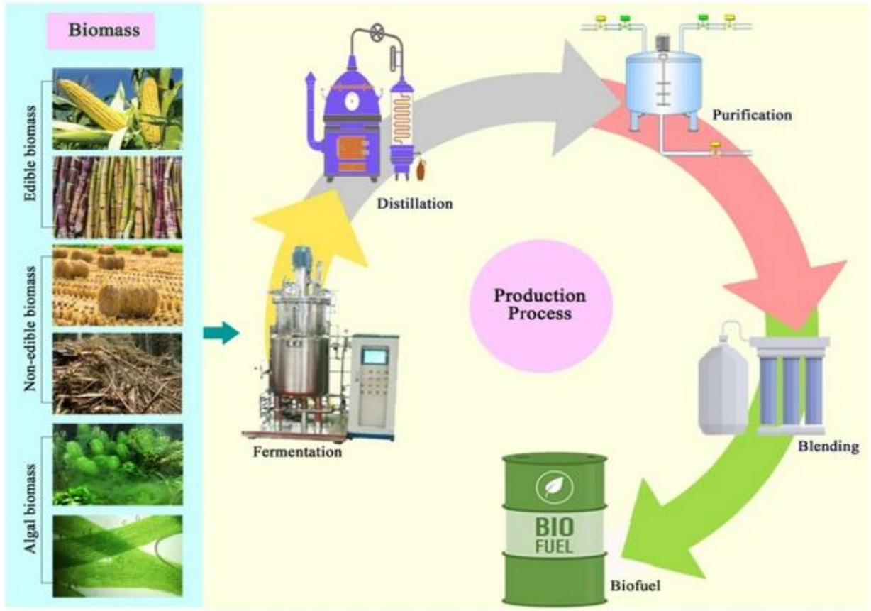
Fig. 1.2: General Biofuel Preparation Process
