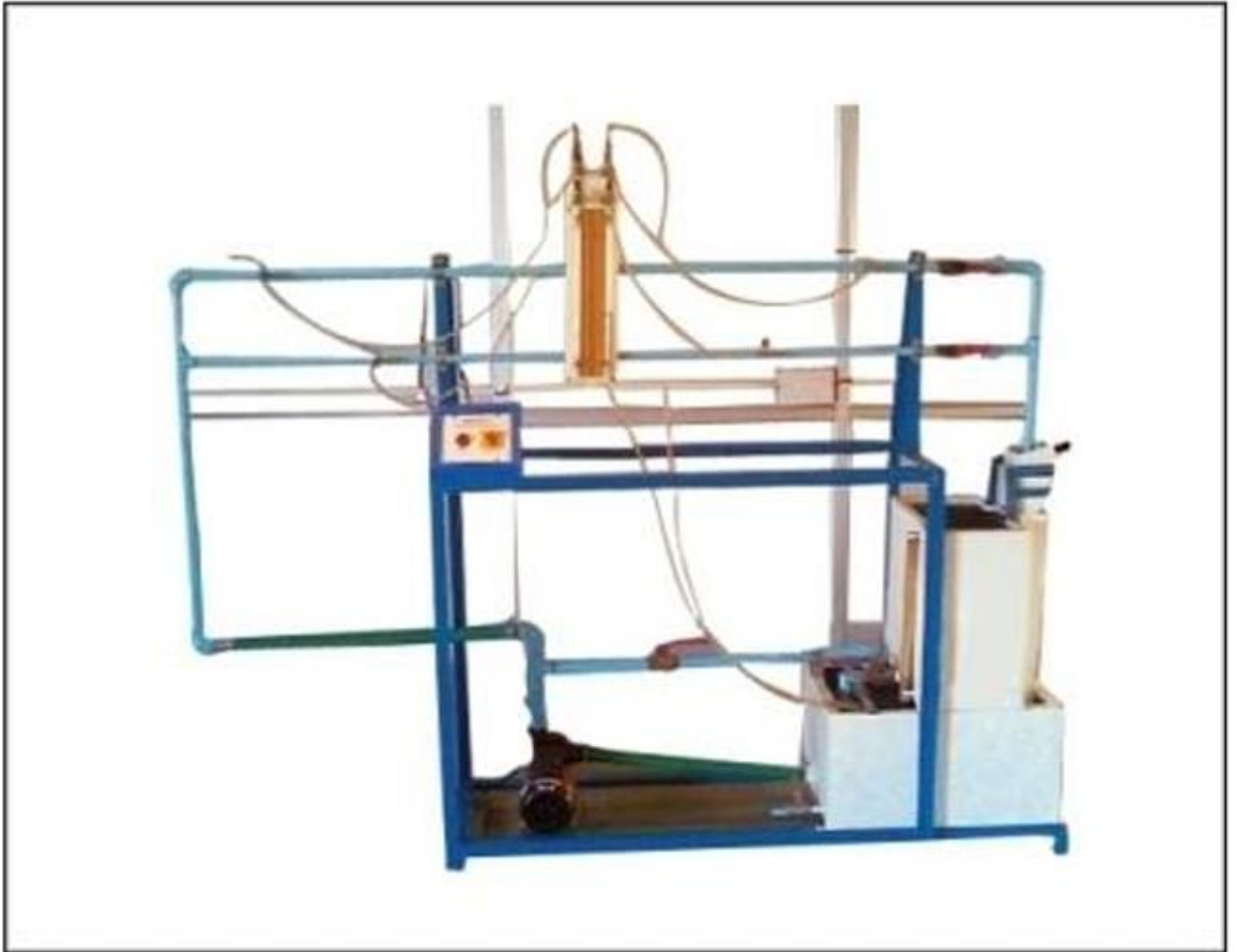
Fig.8.1 Experimental setup for calculation of Darcy's friction factor ' f '
