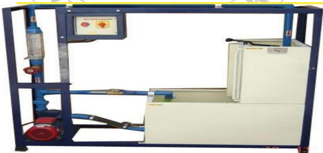
Figure 2.1- Experimental set up of discharge measurement
