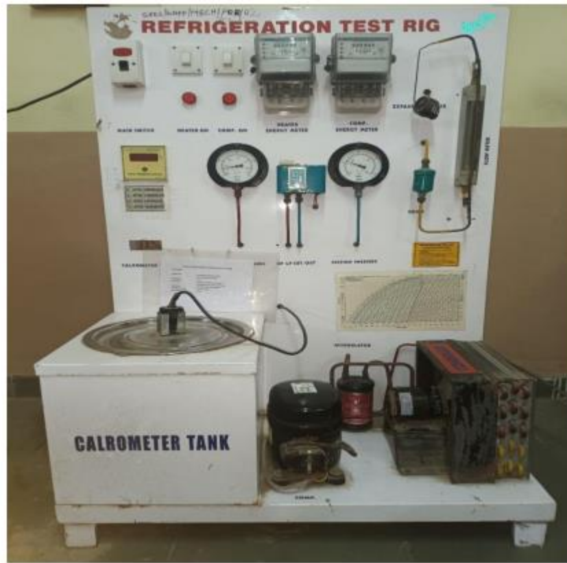
Fig1.5 Vapor Compression Refrigeration System test rig for measurement of pressure, temperature and flow of refrigerent.
