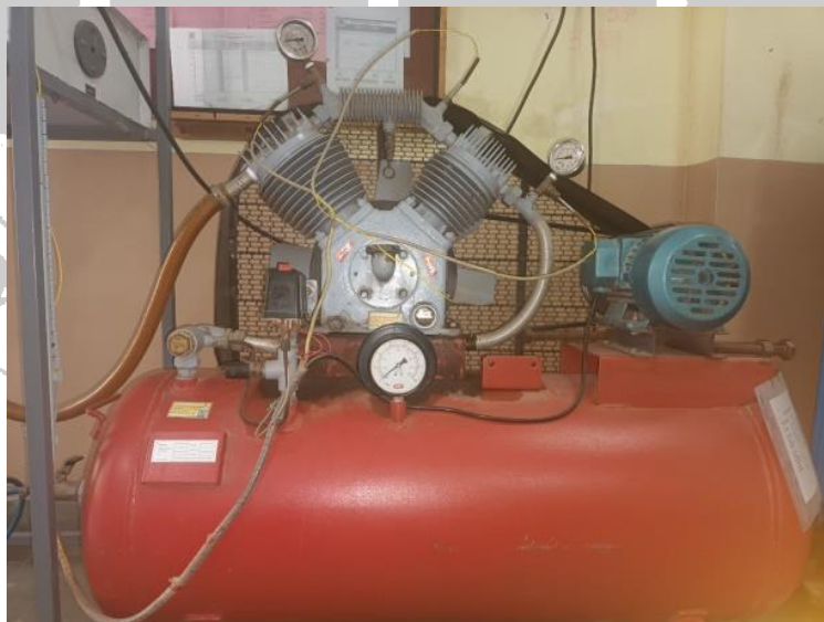
Fig 1.6 Reciprocating compressor test rig for measurement of pressure, temperature and flow of air.
