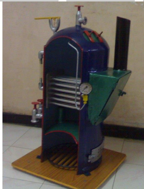
Fig 3.2 Cut section model of Cochran Boiler
