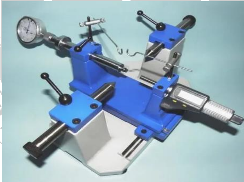
Figure 5.3 Two Wire Method Setup
