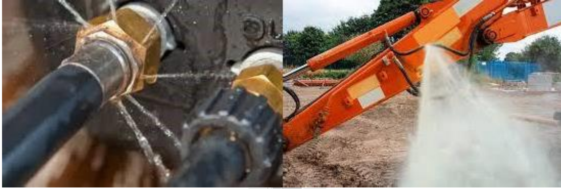
Fig.15.1 Common faults observed in oil hydraulics
